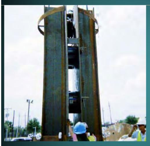
Two 16 MN (3600 kip) O-cells test lateral stiffness of the Cooper Marl (19-21 m depth) on a 2.4 m (8') pile
