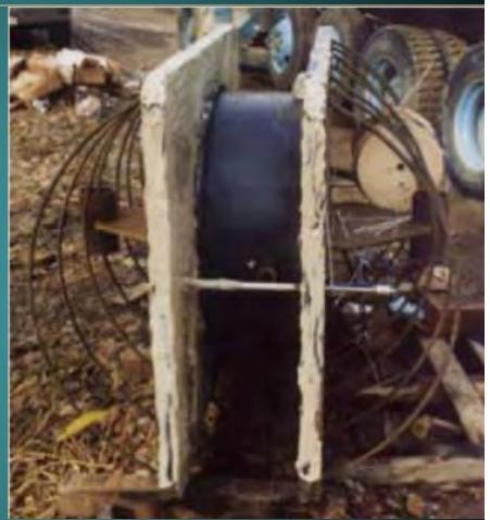
27MN (6000 kip) O-cell used to test a 1.5 m (5') long by 1.2 m (4') diameter rock socket
